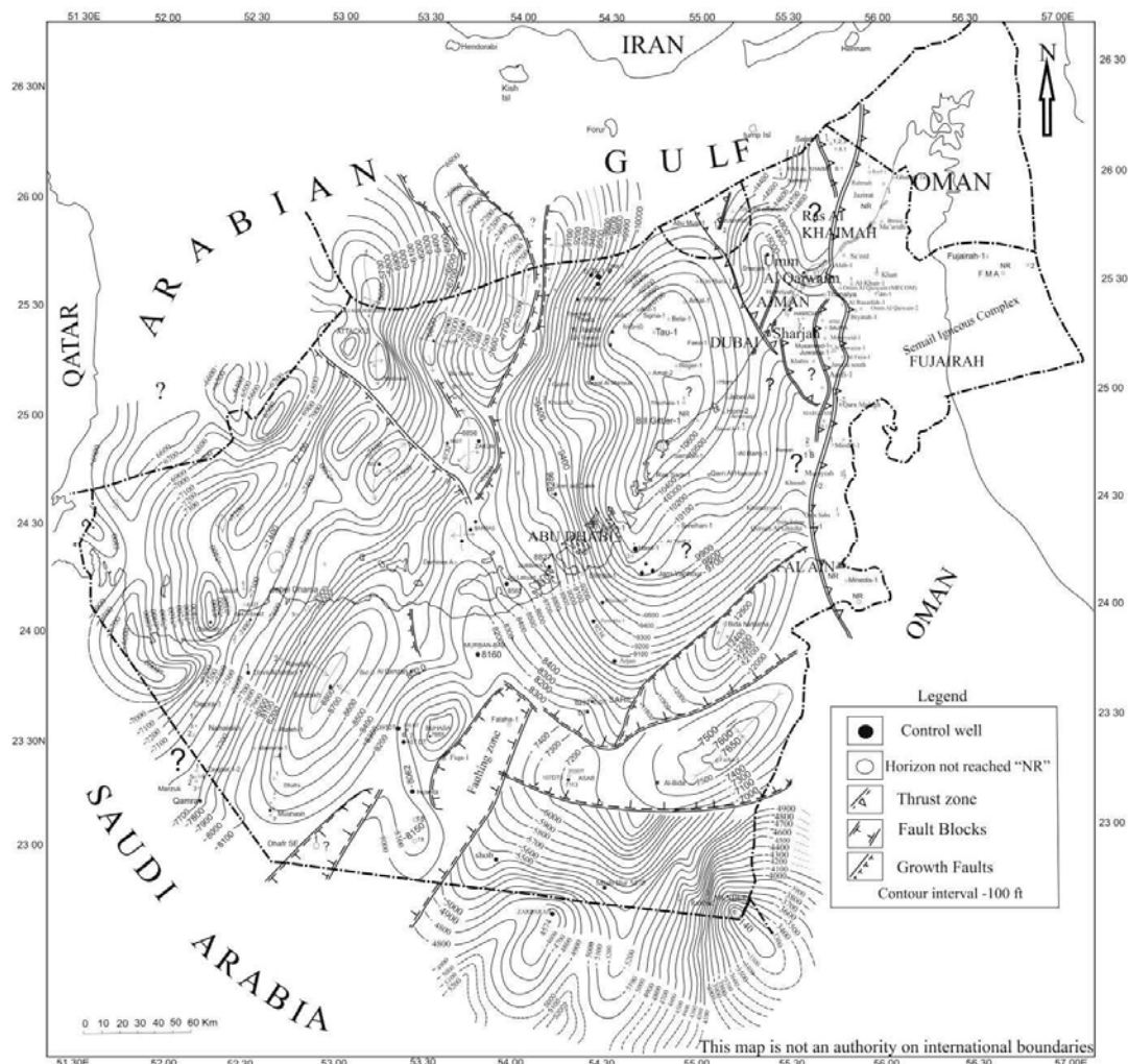
Fig. 7 Structure contour map on the top of the Early Cretaceous / Thamama Group in U.A.E. region.
