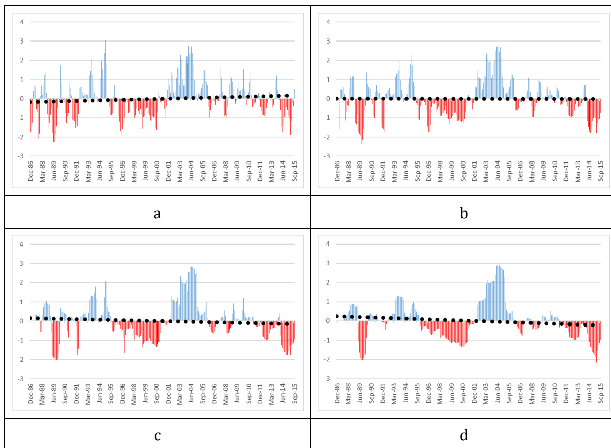
Figure 5. Trends of the standardized streamflow index for station 49: a) 3 months b) 6 months c) 9 months d) 12 months
